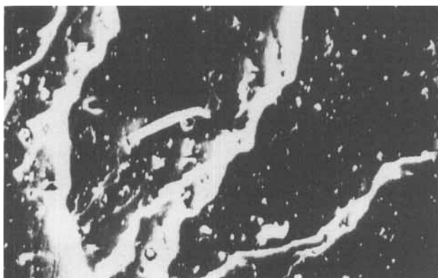
FIGURE 12 SEM fractogram for tensile failure for blend I (100 \times ).
